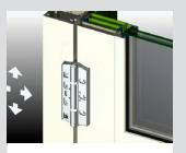
The doors have been designed to accept a heavy adjustable hinge. Screw cover plates removed to show the adjustment screws.
